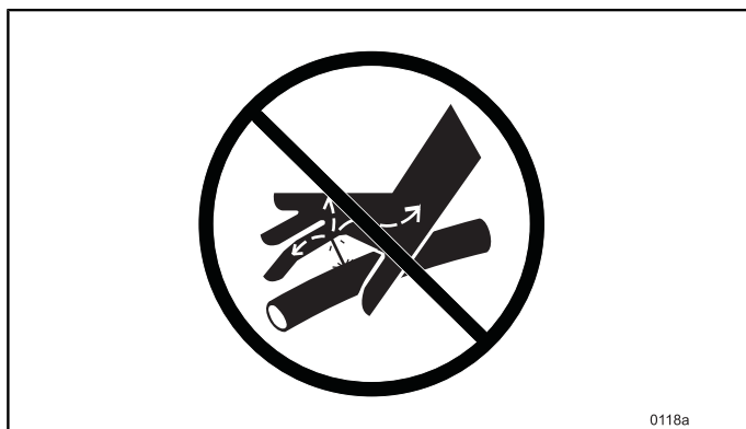
Fig. 83 NEVER use fingers or hands to detect leaks.
