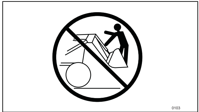
Fig. 30 Do NOT use the loader or the implement to lift or transport people.
