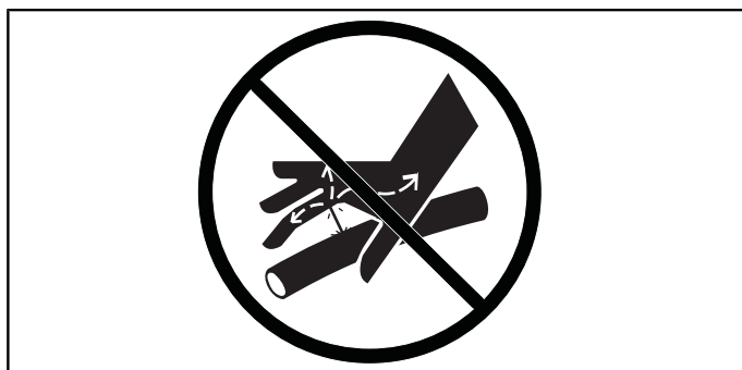
Fig. 18 NEVER use fingers or hands to detect leaks.
