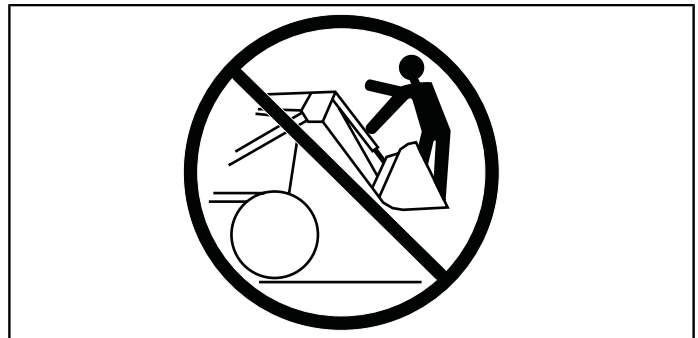
Fig. 67 Do NOT use the loader or the implement to lift or transport people.
