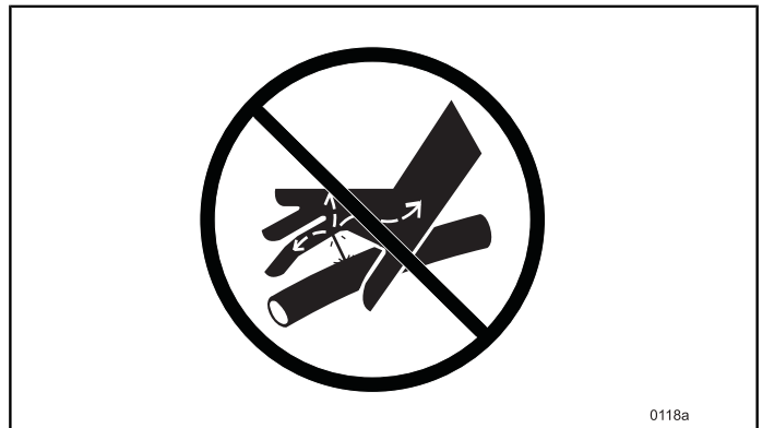
Fig. 43 NEVER use fingers or hands to detect leaks.
