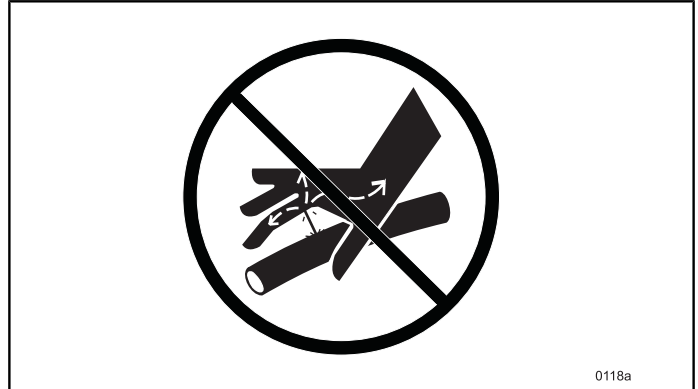
Fig. 85 NEVER use fingers or hands to detect leaks.
