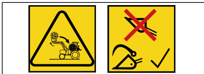
Fig. 70 Only lift loads which can be contained in, and are intended for, the specific implement.
