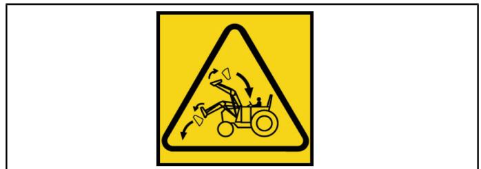
Fig. 32 Keep your eye on the implement, objects may fall backwards onto the operator.
