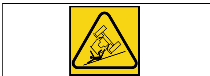
Fig. 35 Crushing and overturning risk
