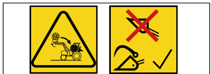
Fig. 41 Only lift loads which can be contained in, and are intended for, the specific implement.
